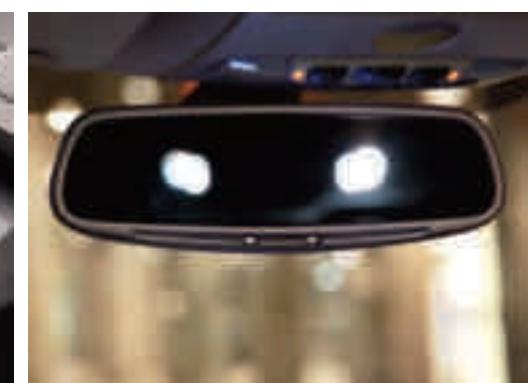
Auto-dimming rear-view mirror A sensor detects harsh lights behind you and dims the mirror. (Standard)
